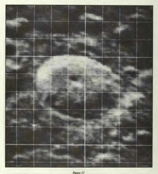
Radar map of the lunar crater Tycho with a resolution of 1 kilometer made with the 3.8-cm (7,750-MHz) Haystack Observatory radar. The grid lines are spaced about 17 km apart. (Courtesy of MIT Lincoln Laboratory, Lexington, Massachusetts, photo no. 242336-1.)
