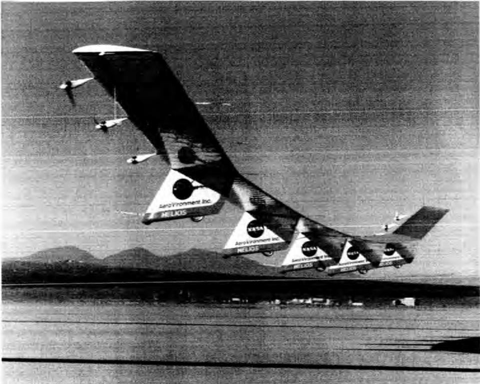
Fig. 4. Helios vehicle being flight tested at Dryden in preparation for its record setting altitude flight in Hawaii. (EC99 45285-5)
