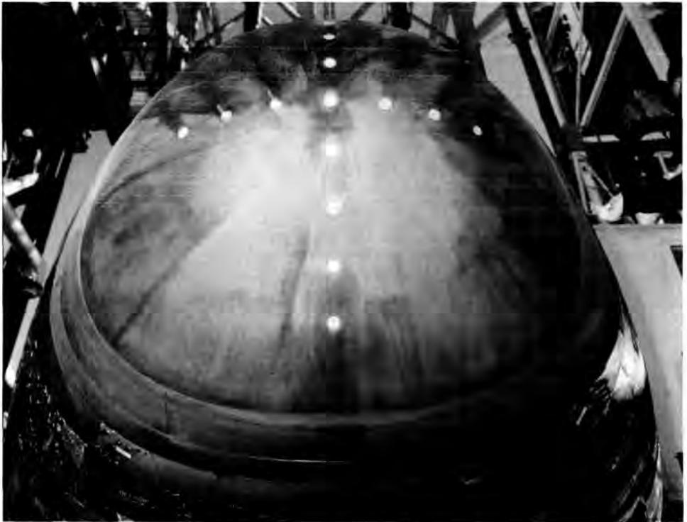
Fig. 6. The SEADS ports are placed in a cruciform configuration on the Space Shuttle Columbia nose as shown in this photo taken after STS-24. (EC86 33311-28)
