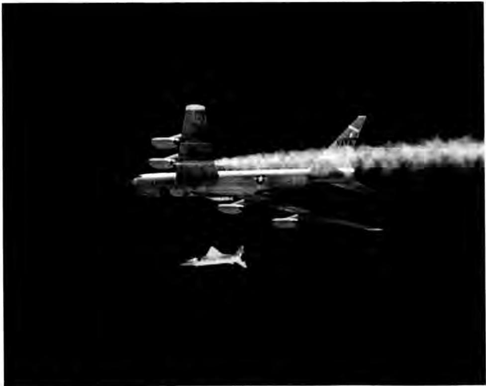
Fig. 6. The X-43 immediately after launch from the B-52 on June 2, 2001.
