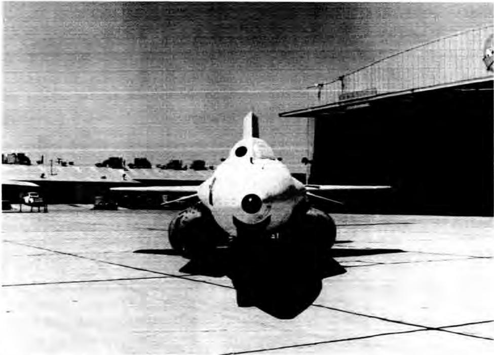
Fig. 2. X-15A-2 in August 1967 prior to the first flight, equipped with the full ablative coating, eyelid, 20-degree dummy ramjet, and external tanks. (E 17339)
