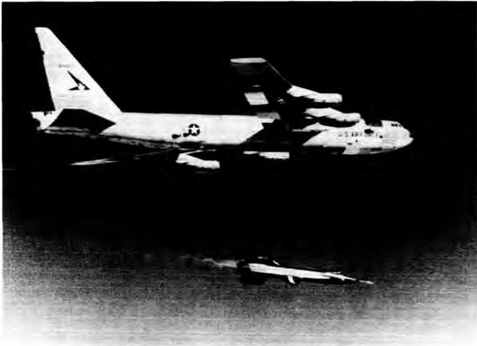
Fig. 4. The number one X-15 just after being launched on June 8, 1959. This is Scott Crossfield's first glide flight flown with the X-15 nose boom, North American Aviation livery, and the XLR-11 engines. (E88-013-15).
