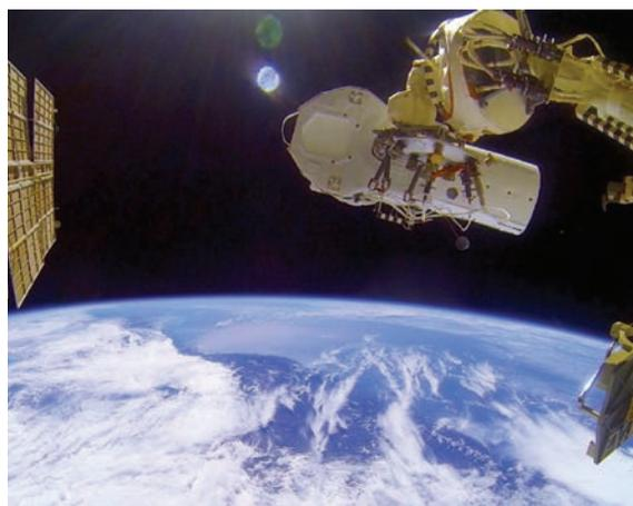
*UrtheCast camera being installed on the Russian Segment of the International Space Station.*
