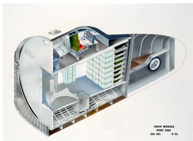
The orbiter's two-story crew cabin contains a flight deck on the top level and living quarters underneath. This cut-a-way view shows the left side of both stories.
