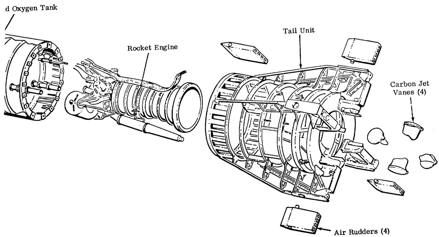
Figure 4-2. Exploded View of Launch Vehicle Structure
