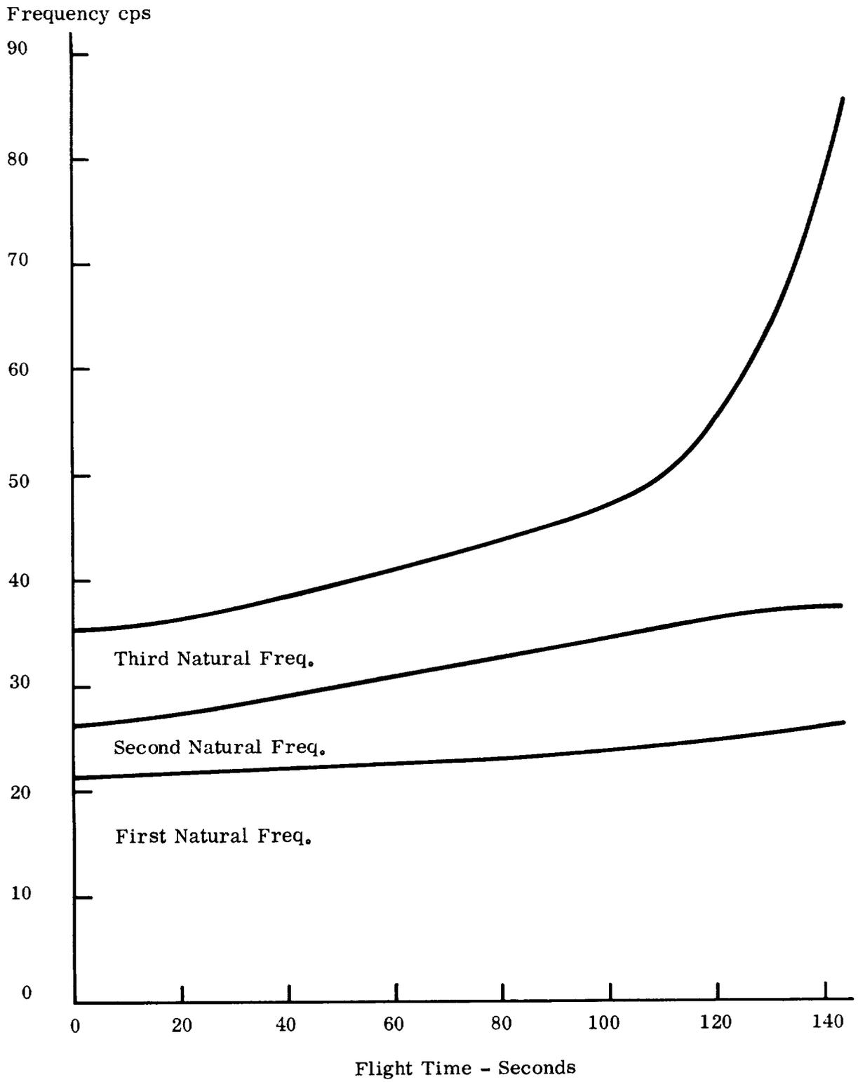
Figure 4-16. MERCURY-REDSTONE Free-Free Longitudinal Natural Frequency versus Flight Time
