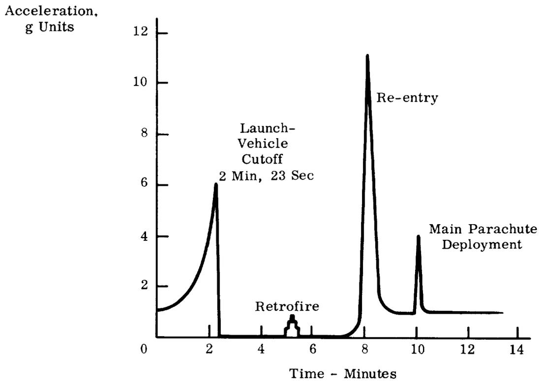
Figure 3-3. Axial Acceleration versus Time, MR-4 Mission
