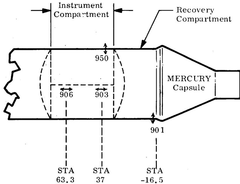
Figure 6-5. Location of Instrument Compartment Vibration Transducers
