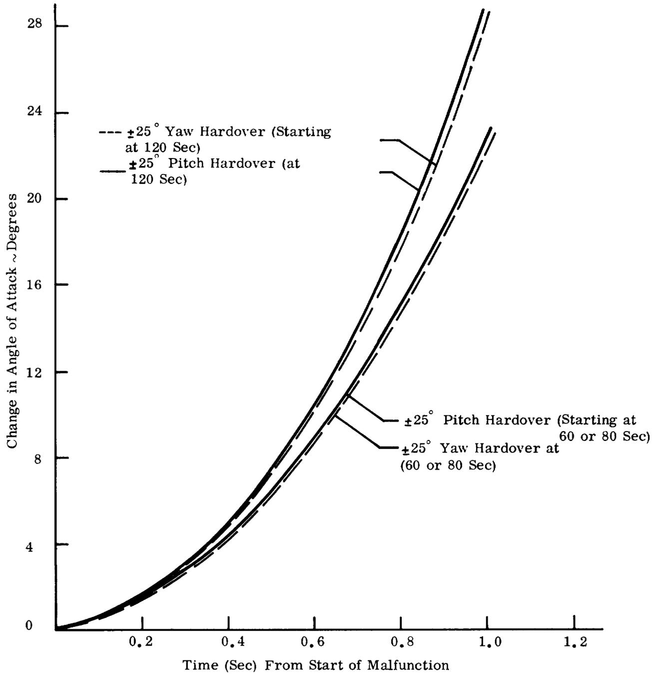
Figure 4-18. Effects of Pitch and Yaw Hardover on Vehicle Angle of Attack (As a Function of Flight Time)
