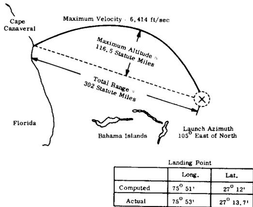
Figure 8-7. MERCURY-REDSTONE MR-3 Ground Track and Flight Profile
