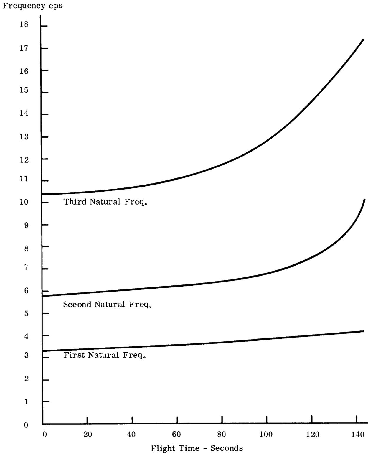
Figure 4-15. MERCURY-REDSTONE Free-Free Lateral Bending Natural Frequency versus Flight Time
