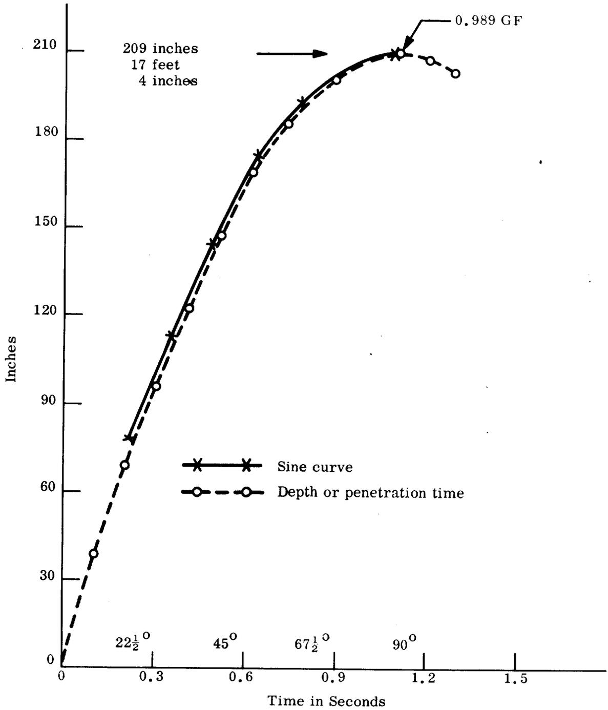
Figure 6-14. Penetration in Inches versus Time in Seconds Showing Close Fit of Sine Curve
