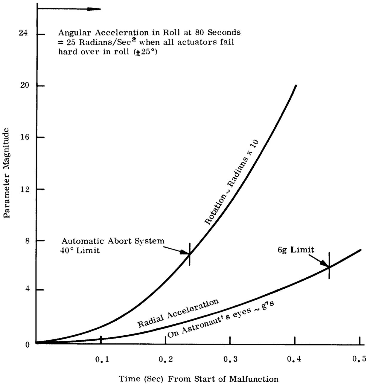
Figure 4-20. MERCURY-REDSTONE Effect of Roll Hardover at 80 Second Flight Time (Worst Case)
