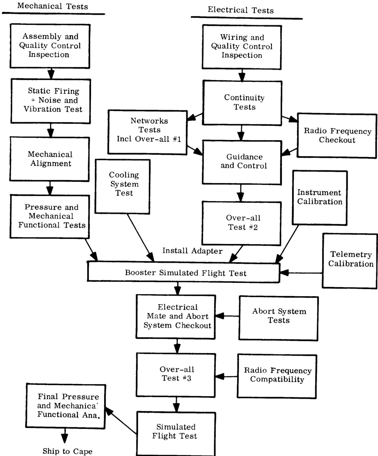
Figure 6-1. MERCURY-REDSTONE System Test Flow Diagram
