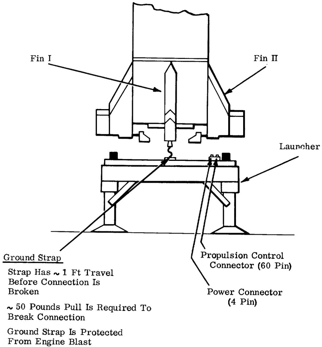
Figure 4-25. Ground Strap Function Just After Liftoff
