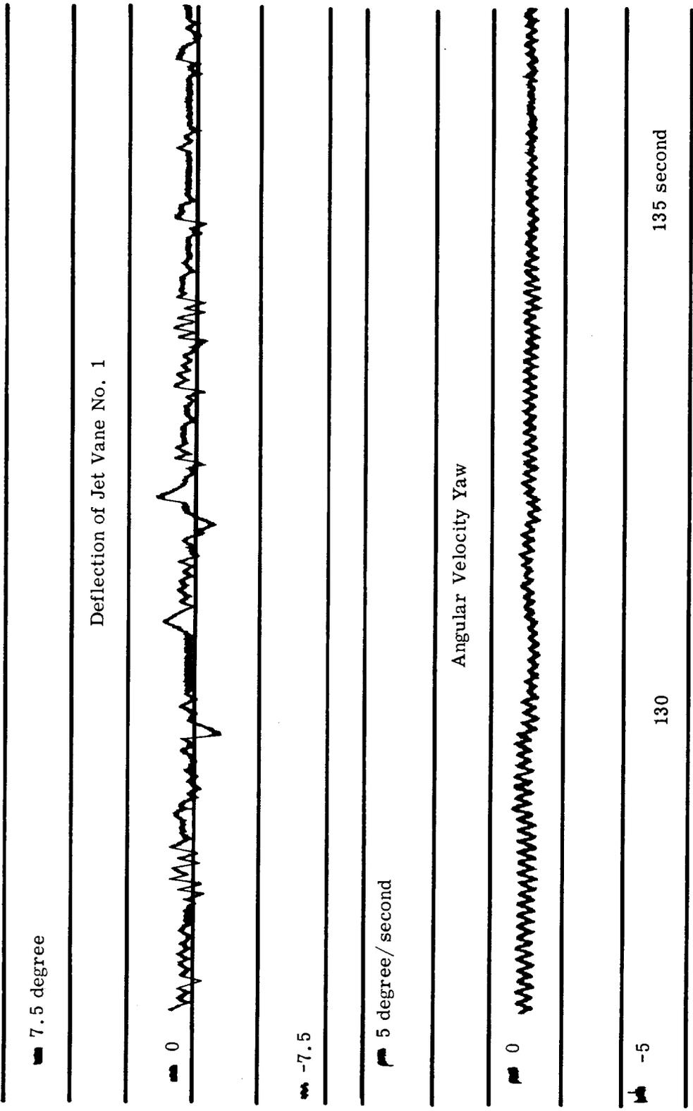
Figure 8-3. Second Bending Mode Oscillations in Yaw Toward End of MR-1A Flight
