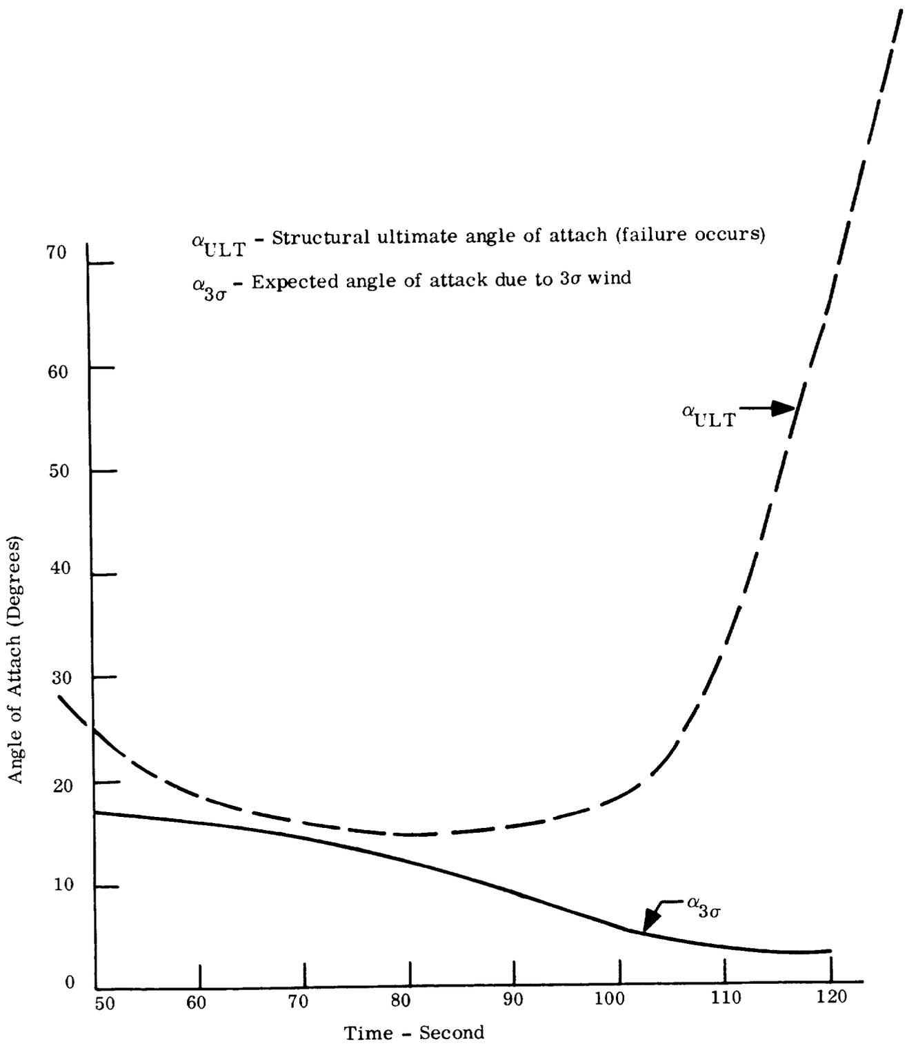
Figure 4-17. MERCURY-REDSTONE Comparison of Angle of Attack versus Time
