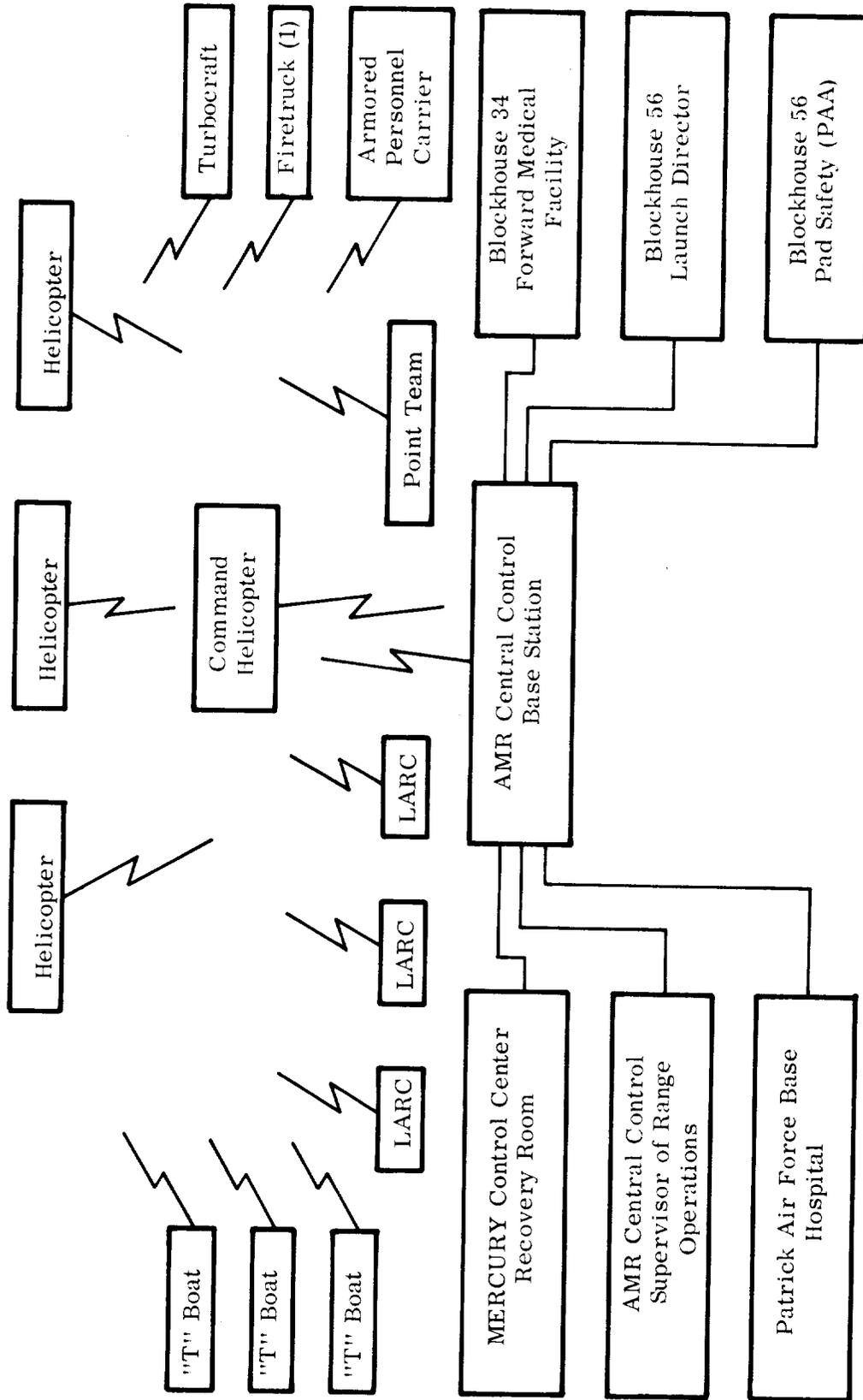
Figure 7-20. Recovery and Rescue Radio Network, High Frequency 30.3
