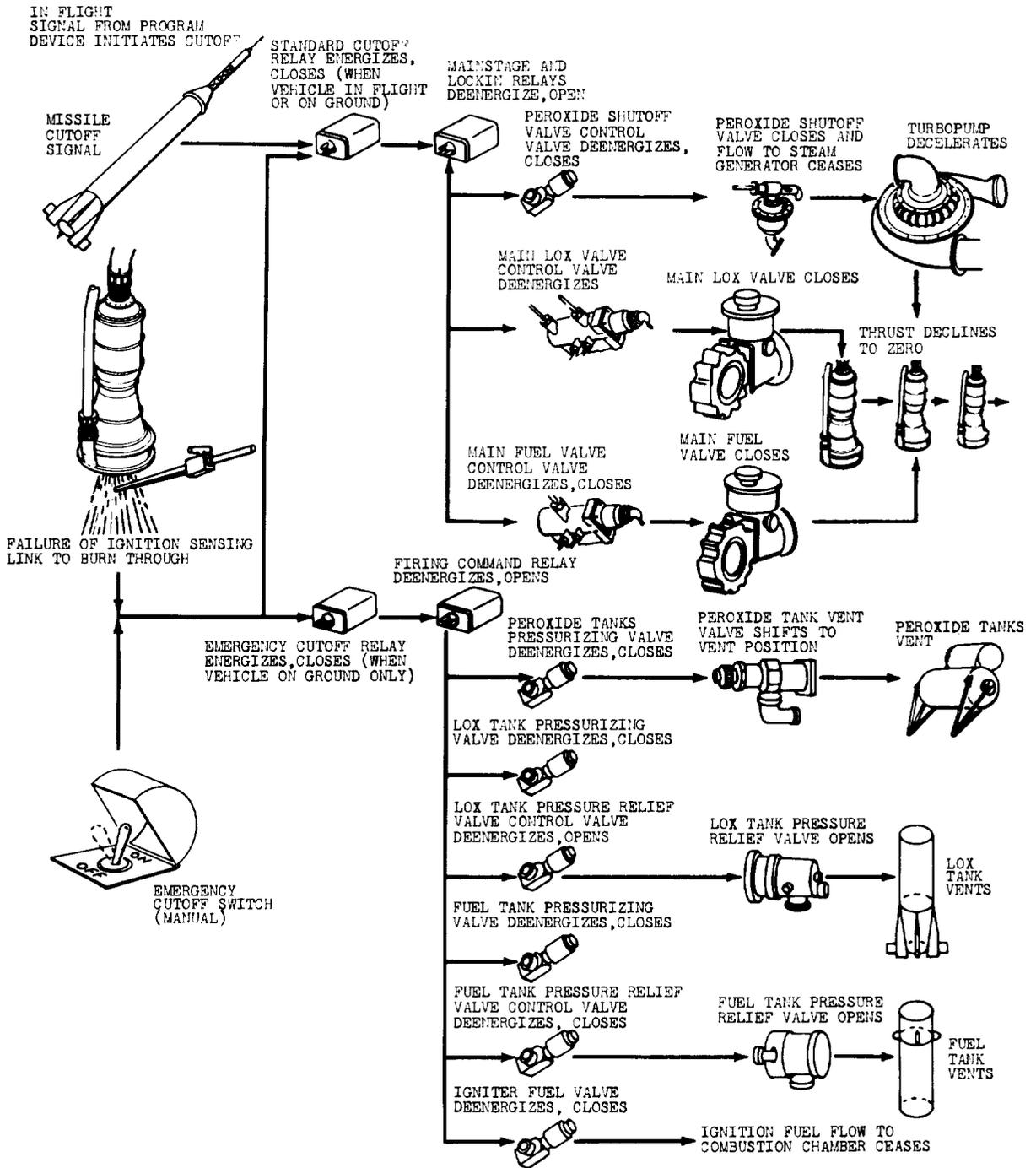
Figure 4-5. Engine Cutoff Sequence Diagram
