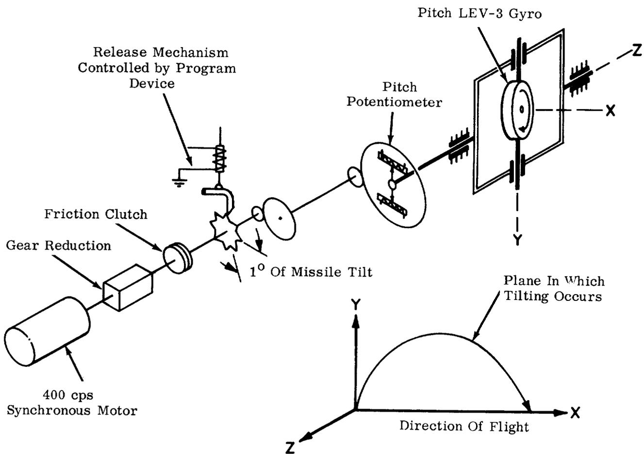
Figure 4-8. Mechanics of Tilting Program
