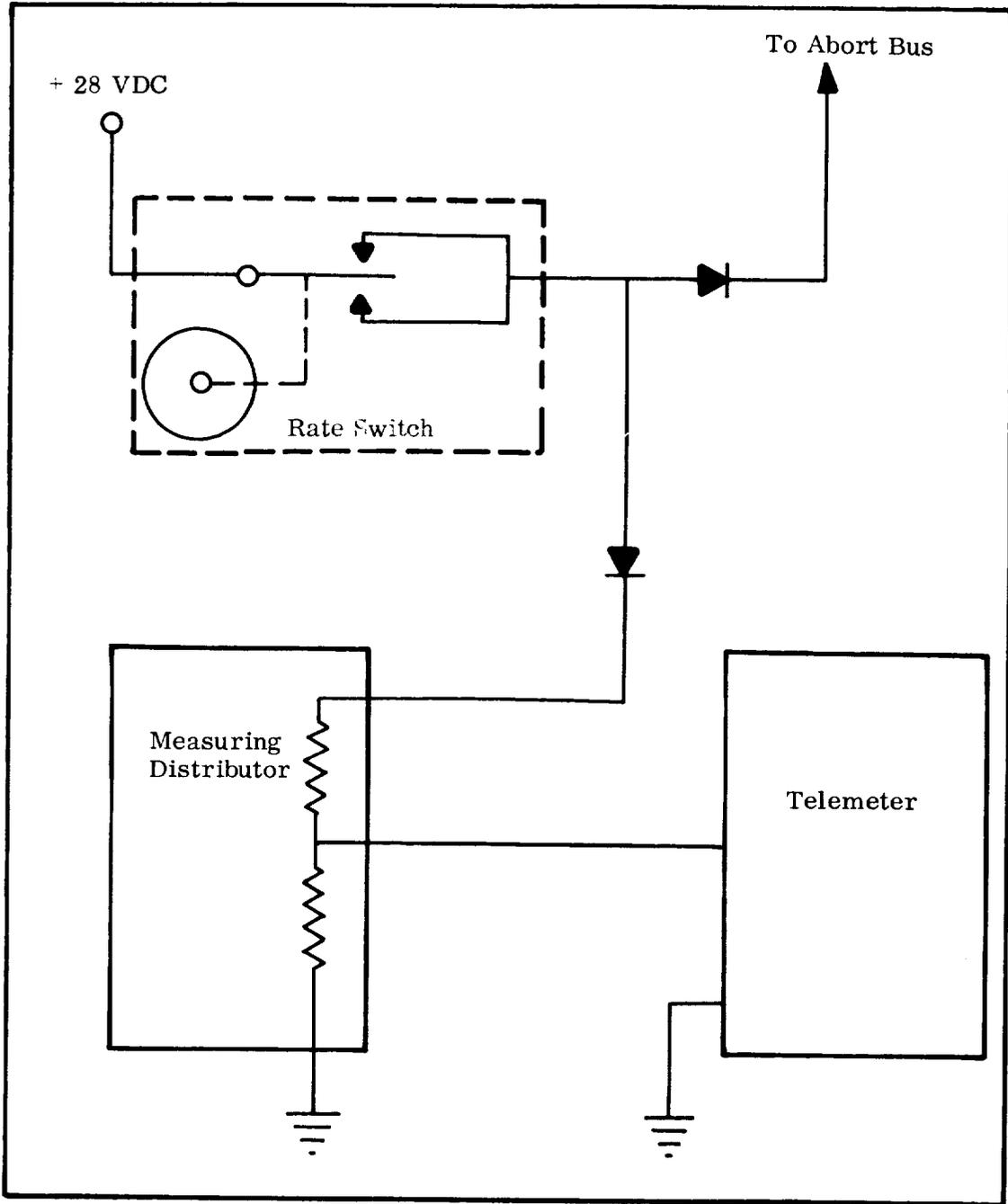
Figure 5-12. Attitude Rate Switch Block Diagram
